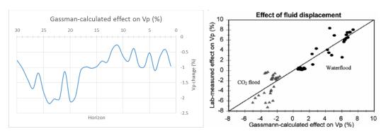
Fig.4.Gassman-Calculated velocity for the Nisku aquifer after one year injection (top) that shows a velocity change maximum to -2%., the second diagram (bottom) is lab and theoretical experiences for CO<sub>2</sub> and water displacement effects on seismic P wave velocities (the CO<sub>2</sub> saturation is many times higher than WASP experience) (Wang,2001).
