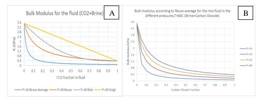
FIG.2. A: Reuss and Voigt average as lower and upper boundary for the fine scale mix and patchy mix fluid. The gray curve was calculated by Brie's fluid mixing model. B: Bulk modulus estimation for different fraction of fluid mix by Reuss average in T=60 C and different pressures
