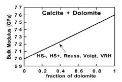
FIG.1. Mixture of calcite and dolomite gives very narrow bounds (Mavko, 2014)
