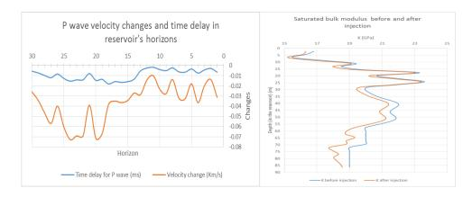
FIG.3. right: it shows P wave velocity change because of  $CO_2$  injection in the each horizon and wave time delay (one way). left: it compares the saturated bulk modulus before and after  $CO_2$  injection in the reservoirs horizons.
