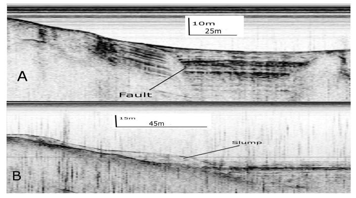
Figure 2- Features observed in Fairbank Lak seismic profiles. (A) Faulting within Fairbank Lake identified by displaced adjacent laminated sections. (B) Slumping observed cross cutting a laminated sediment package. A vertical exaggeration of 2.5 and 3 was used for figures (A) and (B) respectively.
