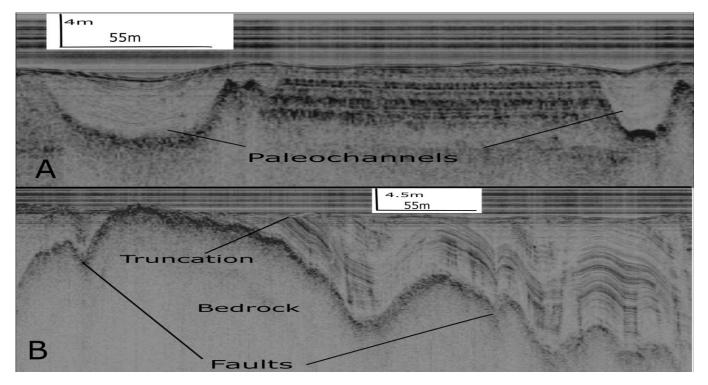
Figure 3- Notable features observed in Lake Vermillion seismic sections. (A) Bedrock overlain by thick laminated sediments truncated at the water-sediment boundary with possible faults indicated. (B) Paleochannels cutting in late glacial sediments in the outlet channel. A vertical exaggeration of approximately 14 and 12 was used for figures (A) and (B) respectively.
