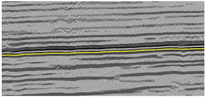
Figure 1. Pre-Stack Time Migration seismic inline section showing a Mannville coal seismic reflector (yellow marker)
