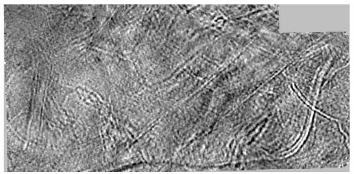
Figure 3. Pre-Stack Time Migration Diffraction Imaging (PSTMDI) horizon slice (corresponding to Figure 2.)
