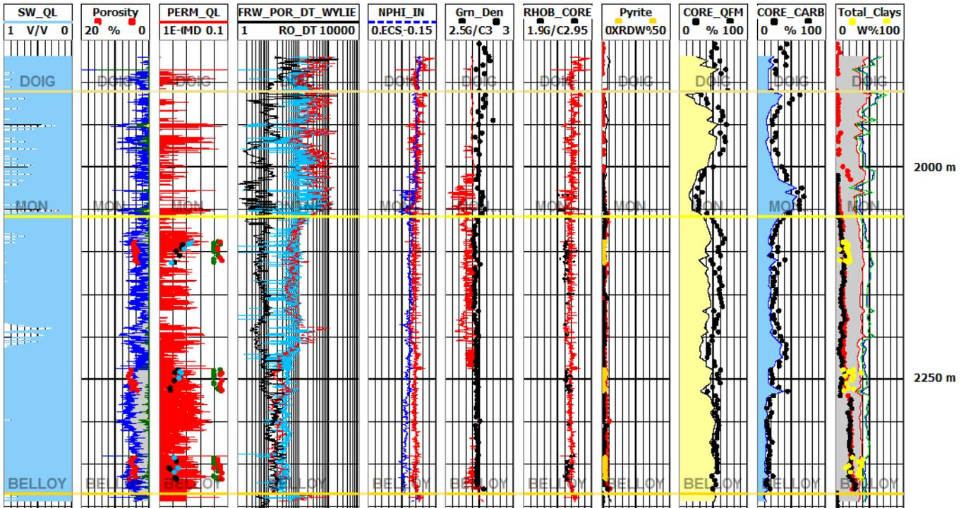
Quick Look Pass 2 with NMR for porosity: Definitely Hydrocarbons (not shown for space limits)
