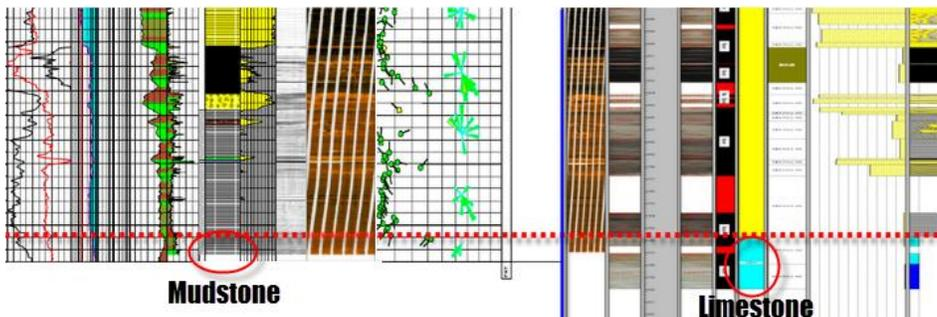
In the image on the left, we see an example where an image log facies interpretation has marked an area as being mudstone while the core description has marked it as limestone. If these interpretations had been made simultaneously, an error such as this would not occur.
