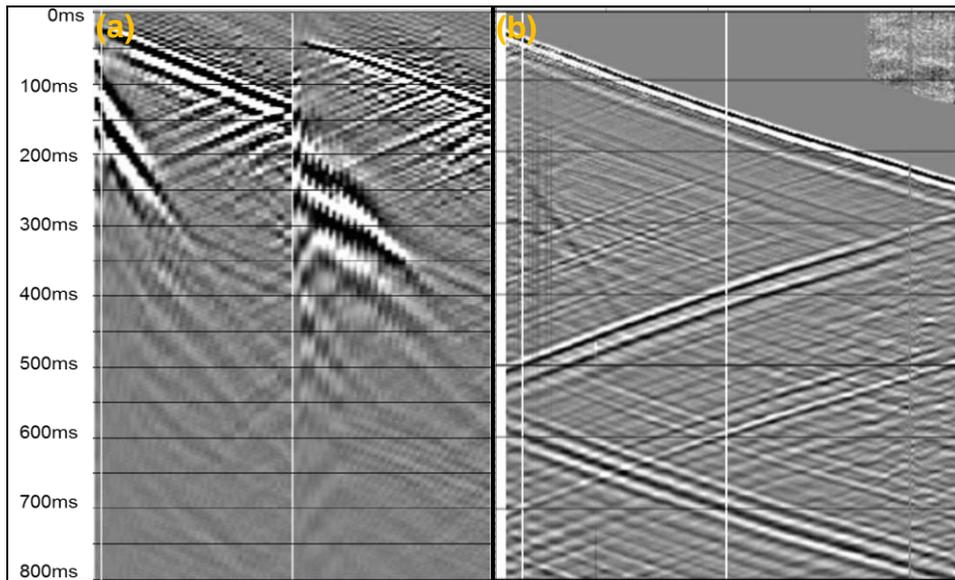
FIG.3. Comparison of DAS-VSP shots and traditional geophone VSP shot. (a) DAS-VSP shots; (b) Traditional geophone VSP shot. DAS-VSP shots show lower S/N, lower resolution, and stronger aliasing.
