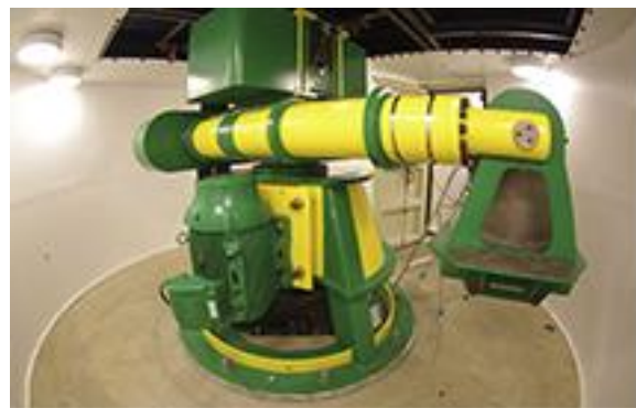
Figure 2 The 50g-tonne beam centrifuge facility
