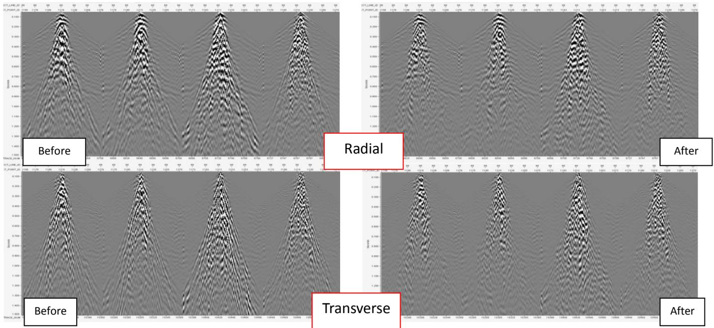
**Figure 2** The radial and transverse components before and after surface wave attenuation and the noise removed
