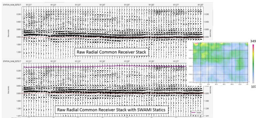
**Figure 5** Application of receiver shear statics derived from the near surface model and map of calculated values
