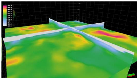
**Figure 4** The near surface Vs velocity model after smoothing
