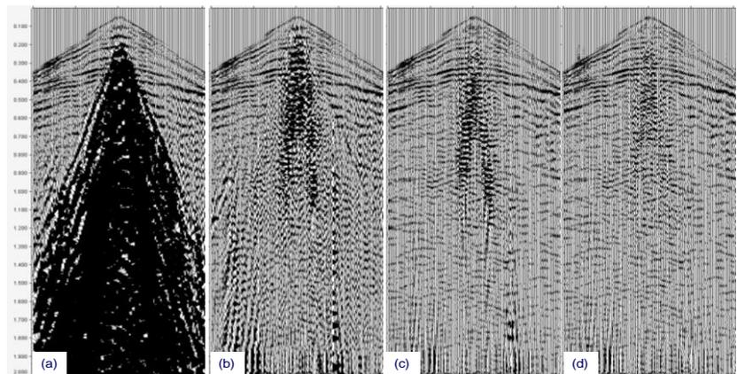
**Figure 1: Oil sands shot gathers. (a) raw data; (b) after SWAMI noise attenuation; (c) cascaded with non-uniform coherent noise attenuation; (d) after additional noise attenuation.**
