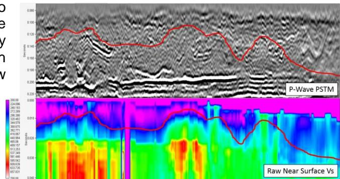
**Figure 3** Comparing the raw  $V_s$  velocity field to the shallow P-wave PSTM section. Similarities at this early state can be noted.
