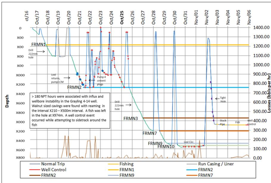
Figure 2: Composite of Bit Depth By Time With NPT and Losses (can be modified as per NPT type)
