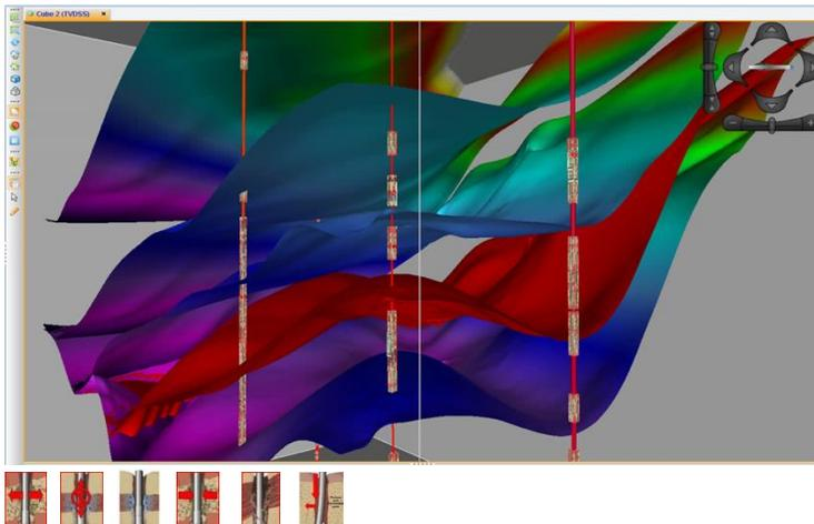
Figure 1: Drilling non-productive events mapped into the sub-surface framework mode
