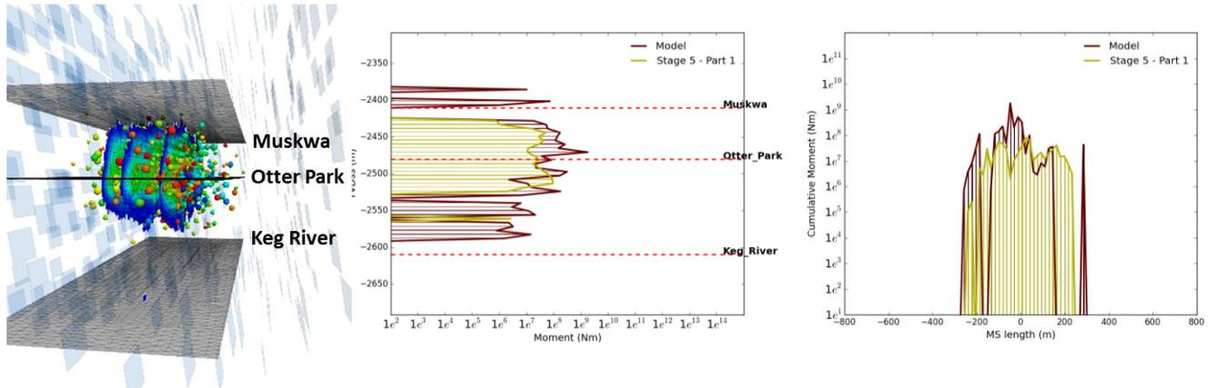
Figure 2. Perspective view of primary fractures and synthetic microseismic (left). Depth (center) and lateral (right) distribution of moment release from the model (red) and observed (green)
