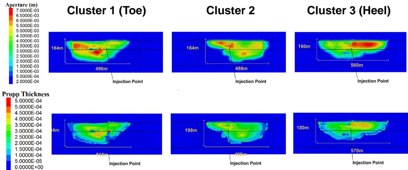
**Figure 5. Primary fracture planes for the three clusters showing aperture (top row) and proppant thickness/concentration (bottom row).**
