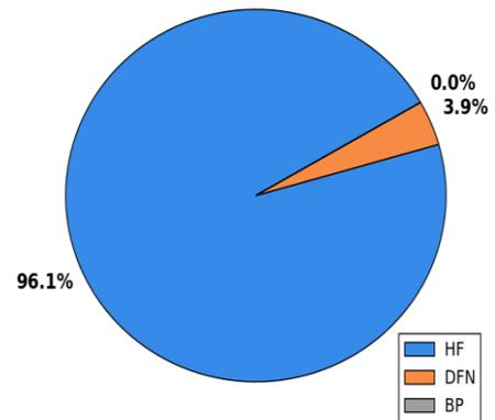
Figure 4. Percentage of the fracturing fluid in different portions of the fracture network.
