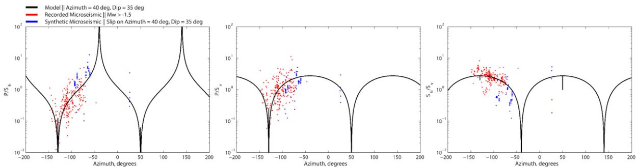
**Figure 3:** Observed amplitude ratios plotted against theoretical values for a double-couple source with an azimuth of 40 degrees and a dip of 35 degrees. Black lines represent theoretical radiation pattern for best fit fault plane, red dots are reported values from the events. Blue dots are values from the synthetic microseismic generated from the geomechanical modeling result. Azimuth is measured relative to grid north, and represents the direction from source to sensor.
