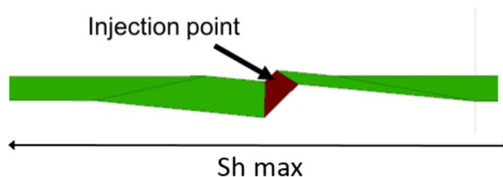
**Figure 4:** Geomechanics fracture geometry with an oriented pre-existing fracture (red) that turns into a primary tensile fracture (green) away from the injection point.
