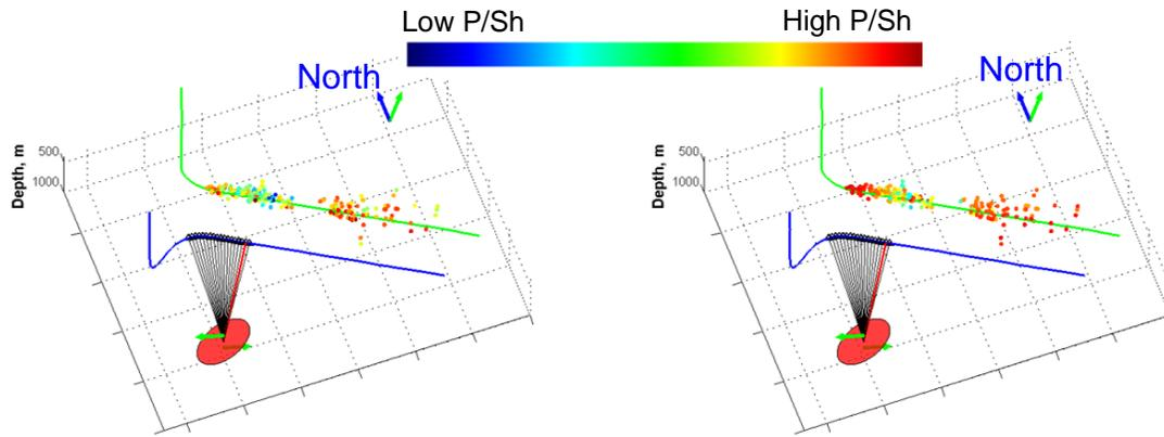
**Figure 2:** Computed P/Sh amplitude ratios (left) and theoretical ratios (right) for the high magnitude event set. Event are colors by P/Sh ratio, and the computed mechanism is illustrated by the red plane. Grid spacing is 1000 meters.
