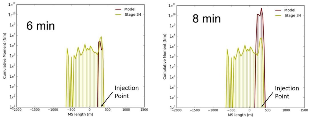
**Figure 5:** Distribution of cumulative moment for an example stage (stage 34, in yellow) and the modeled result (dark red) during the start of injection. Modeled result shows the moment distribution after 6 minutes of injection (left), and again after 8 minutes of injection (right). Note the large increase moment near the injection point, reflected by the model.
