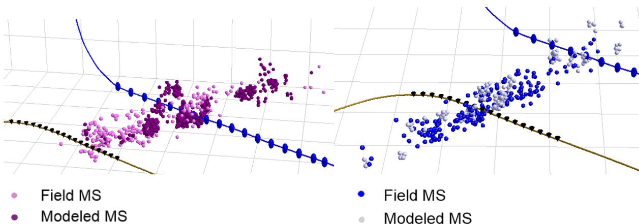
**Figure 2** Comparison of synthetic and field microseismic data for Stage 32 (left) and Stage 34 (right).
