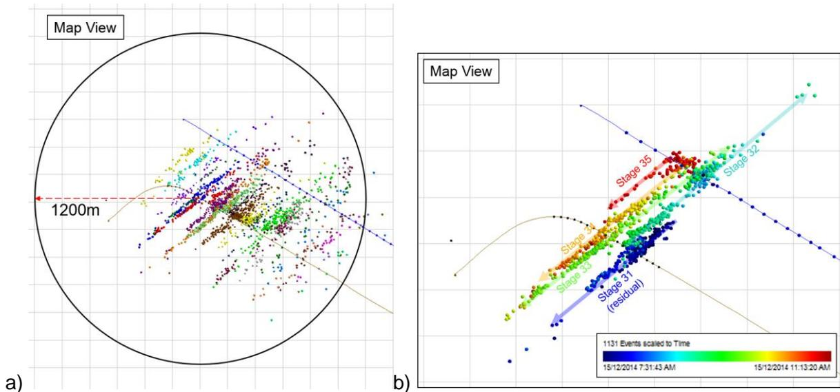
**Figure 1.** a) Plan view of the microseismic data b) Plan view of the microseismic data illustrating varying degrees of asymmetry over stages 31-35.
