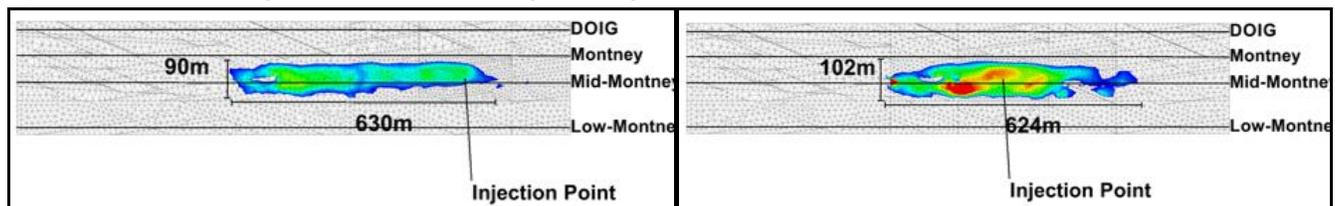
**Figure 5** Effective proppant placement ( $1.0\text{kg/m}^2$ ). a) Asymmetric fracture growth. b) Symmetric fracture growth.
