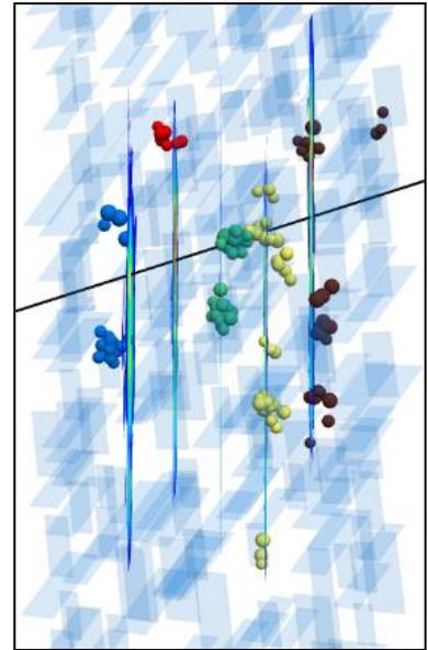
**Figure 3. Asymmetric fractures from multiple perf clusters.**
