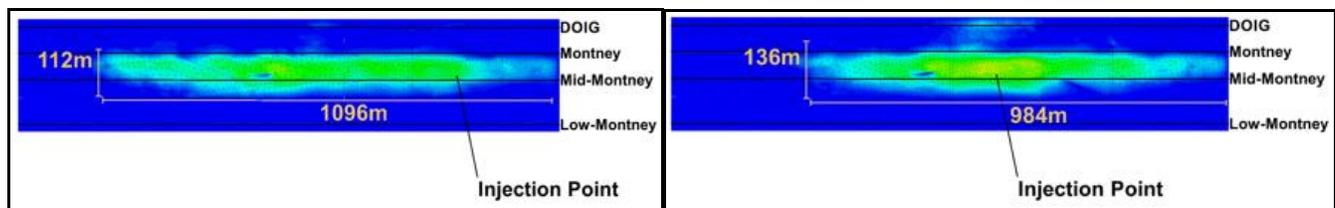
**Figure 4.** Hydraulic fracture extent. a) Asymmetric fracture growth corresponding to Stage 34. b) Symmetric fracture growth corresponding to Stage 32.
