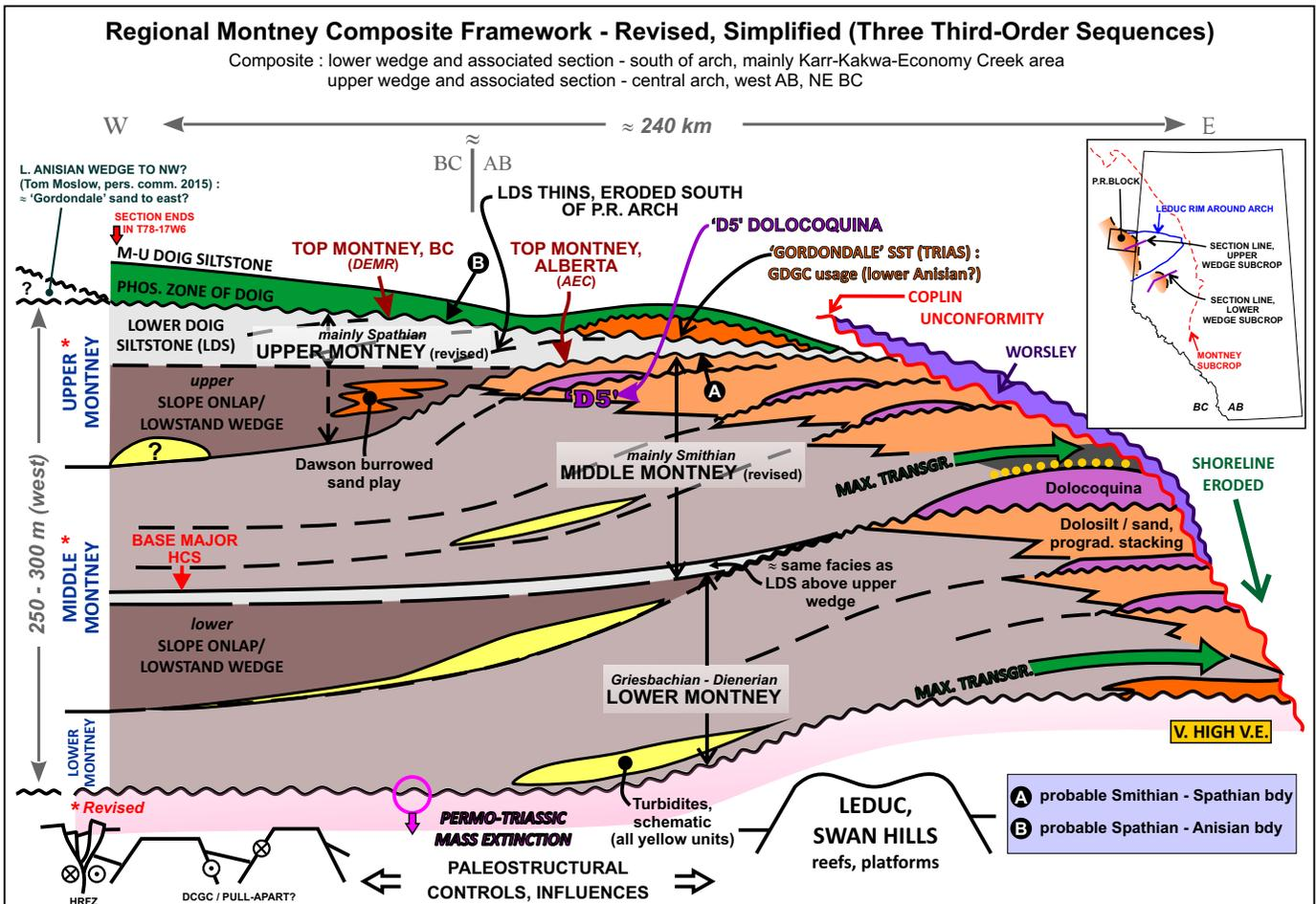
**Fig. 2** Schematic regional Montney composite stratigraphic and sequence framework, using revised subdivision nomenclature based on three Third-Order sequences, and showing general relationships for lower and upper lowstand / slope onlap wedges.
