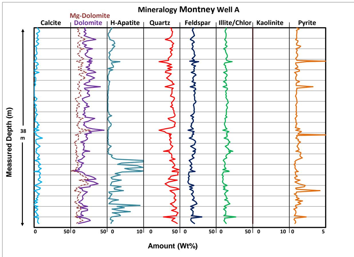
**Figure 1: XRF Calculated Mineralogy Logs From Core. Continuous colored curves show XRF calculated mineralogy.**
