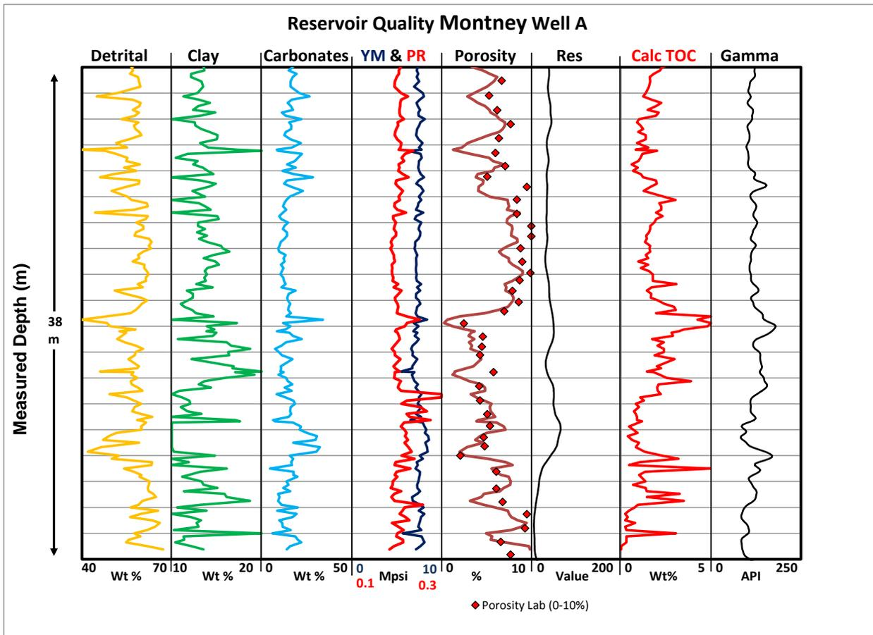
**Figure 2: XRF Reservoir Quality Logs From Core. Continuous colored curves show XRF calculated data for mineral groups, mechanical properties, calculated porosity and TOC. Wireline log GR and resistivity along with lab measured porosities (red diamonds) are also displayed.**
