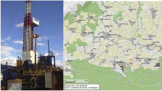
**Figure 1: Left-GRT1 borehole deeping at 2580m, with the openhole at 1922m during the hydraulic stimulations of April 2013 and June 2013 (5000 m3 injected). Right-The surface seismic networks including 18 sensors (Red, blue and white squares) sampling at 100,**
