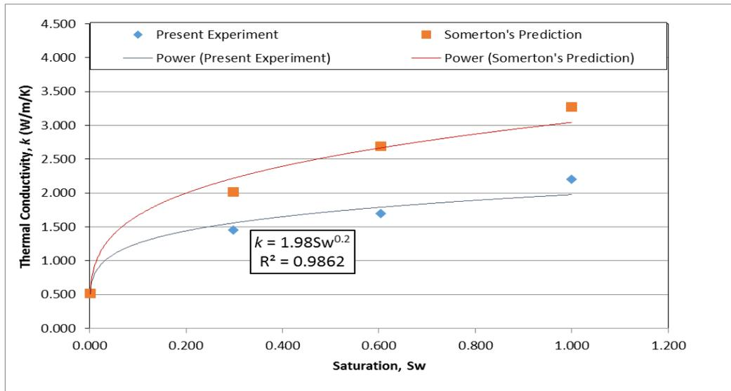
Figure 1: Thermal Conductivity of Oil Sands at Various Saturations of Water Compared with Prediction of Somerton (1992)
