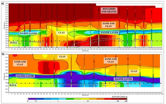
**Figure 2** Resistivity profiles derived from TDEM soundings. a) Profile P1-2 located in area 1. b) Profile P2-4 in area 2. Both geoelectrical sections display a saline layer with resistivity values lower than 1  $\Omega$ .m.
