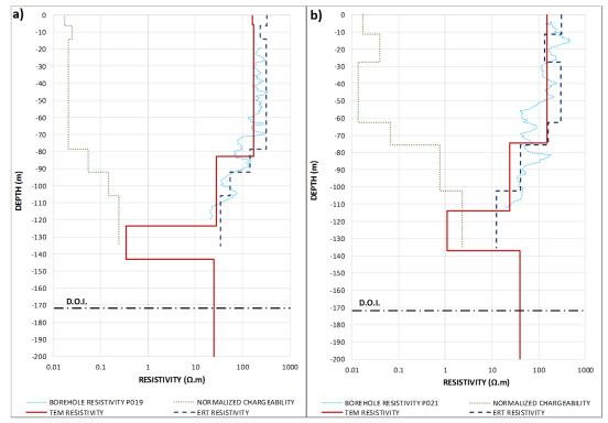
**Figure 1** Comparison of resistivity values from borehole logging, ERT and TDEM. The normalized chargeability is also included. a) and b) are for the borehole P019 and P021, respectively.
