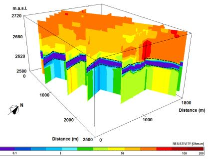
Figure 3 A 3D visualization of the resistivity distribution in area 2.
