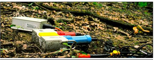
Figure 2 shows a compact cableless node with a connected battery and 3C sensor.
