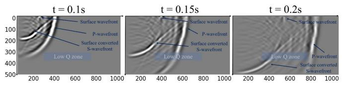
Figure 3 Snapshots for x component wavefield in localized attenuation model
