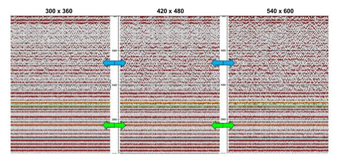
If the prime zone of interest was a gentle structural roll-over at a major reflector such as indicated by the green arrows, then the least dense model is sufficient. The higher dollar cost and environmental disturbance of the two models to the left would not gain significant interpretability for such a prospect.
