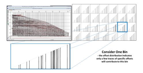
A typical example of signal and noise variations with offset is provided by a CMP super-gather from existing data (top left in the figures above and below). The geometric 3D model indicates which traces of which offsets will combine in each bin. Then only traces matching the modelled offsets are selected and stacked to form one trace for that bin.
