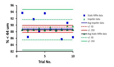
Graph 2. The actual data entries of 10 analyses for each method in addition to the average, average±SD and average±2SD are shown above. Both series were overlaid for a better visualization of the precision difference. As demonstrated the error of subsampling is much larger in the riffle method. Note that the average of both techniques are nearly identical.
