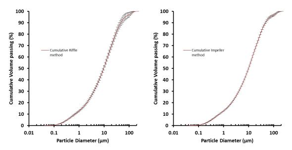
Graph 1. Right and left show the cumulative volume percentages of impeller and riffle methods respectively. Findings demonstrate the error of subsampling is much larger in the riffle method than impeller method.
