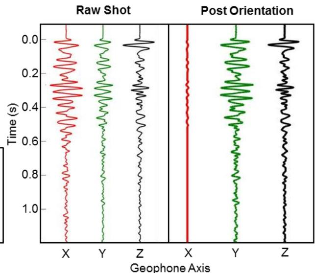
Figure 3. Example Orientation shot. Raw Shot shows data prior to rotation from resulting hodogram analysis. Post orientation has optimized maximum signal in Y vs minimum signal in X. Hodogram: Yellow shows cross-plotted horizontal traces with least squares linear fit in black.
