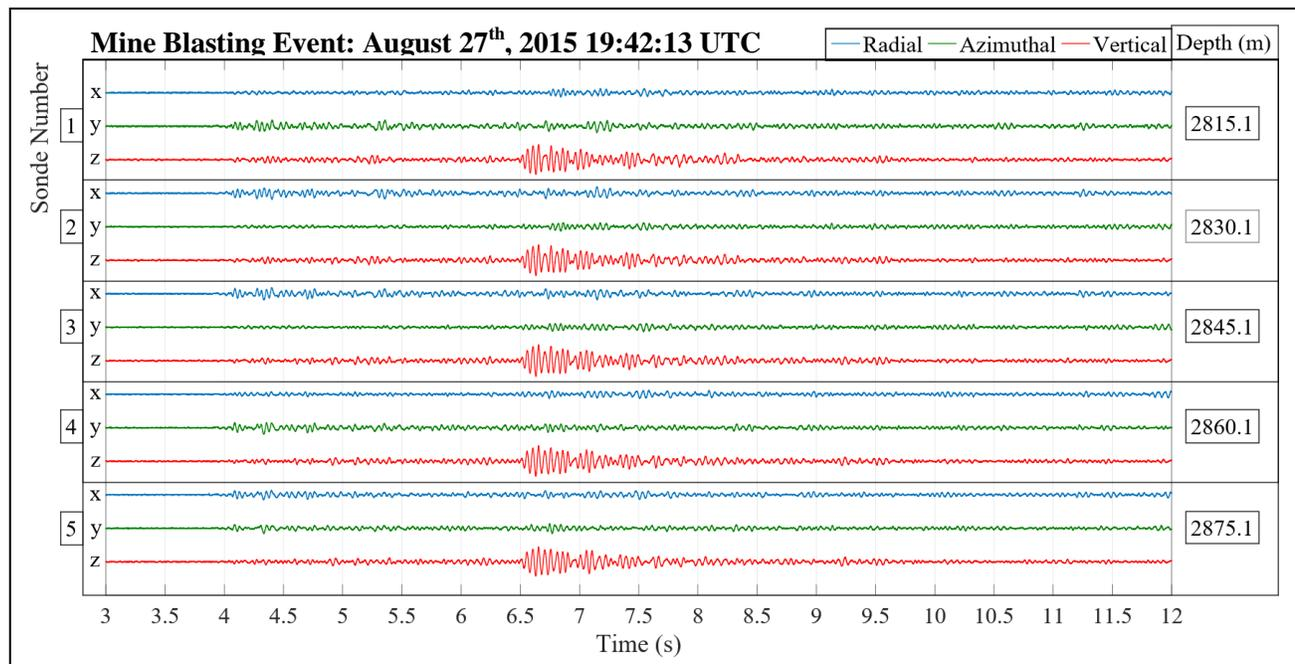
Figure 4. P-wave apparent moveout (upward): 12000 m/s. S-wave apparent moveout (upward): 8600 m/s. S-wave appears strongly only on vertical component. Associated with local mine blasting event.
