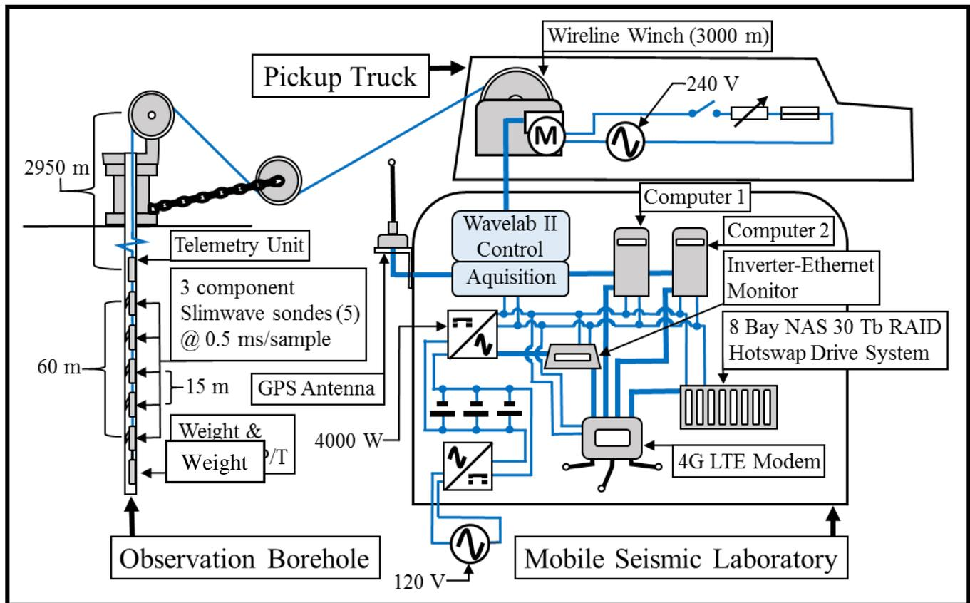
Figure 2. Microseismic Monitoring, Technical Layout. System depicted in deployed configuration. Battery backup ensures uninterrupted monitoring. Precise timing provided by GPS antenna. NAS drive system ensures no data lost. Remote computer operation and data retrieval possible through cellular uplink.
