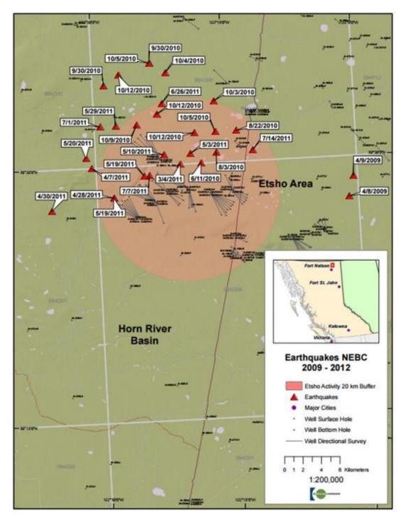
Figure 2. Major seismic events recorded near hydraulic fracturing operation sites in British Coulombia, Canada, event locations and drilling pad locations within 10 km radius shaed circle (source: BCOGC, 2012).
