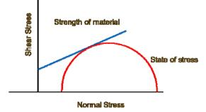
Figure 1. Mohr Coulomb space relating stress to material strength and failure conditions.
