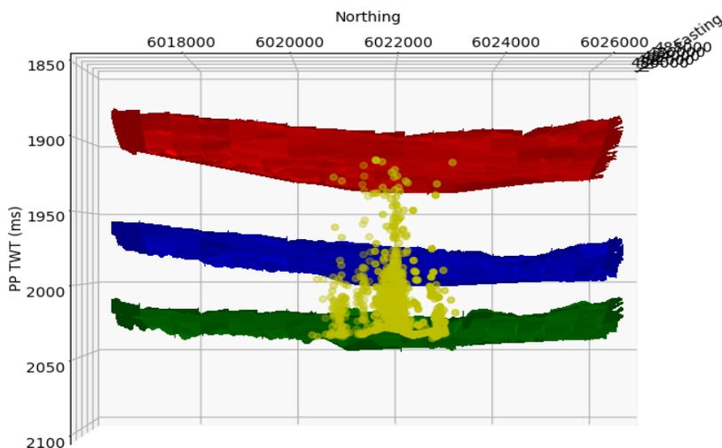
Figure 3 Microseismic events in terms of P-P time plotted against picked horizons Ireton (red), Swan Hills (blue) and Gilwood (green).
