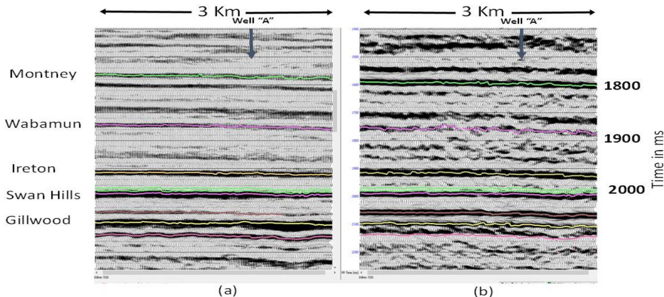
Figure 2. PP (a) and PS (b) seismic data in PP time, showing events used for registration of PP and PS arrival times.
