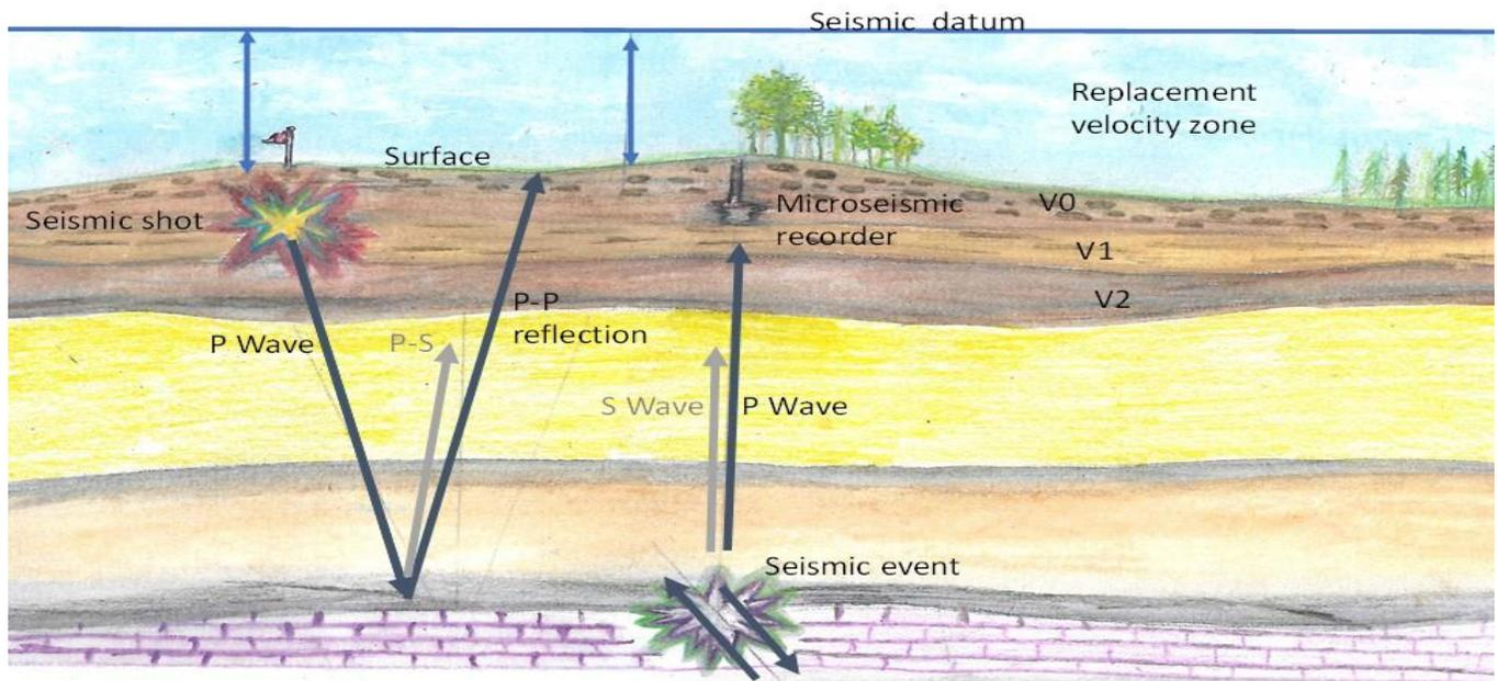
Figure 1. Illustration of the relationship between reflection seismic data and microseismic recording. Reflection seismic data is corrected to an artificial datum, above the highest elevation. The dark arrows represent PP (reflection) and direct P-wave, the gray arrows represent PS (reflection) and direct S-wave (microseismic). The reflection seismic data is time-adjusted downward to match the microseismic data.
