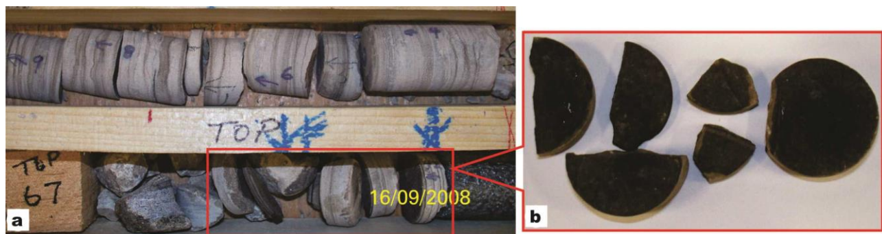
Figure 4. Short core from Station 67, Cruise 82034, Hudson Strait. a: parts of the short core; b: view of cross section from part of top core showing the black shale layers
