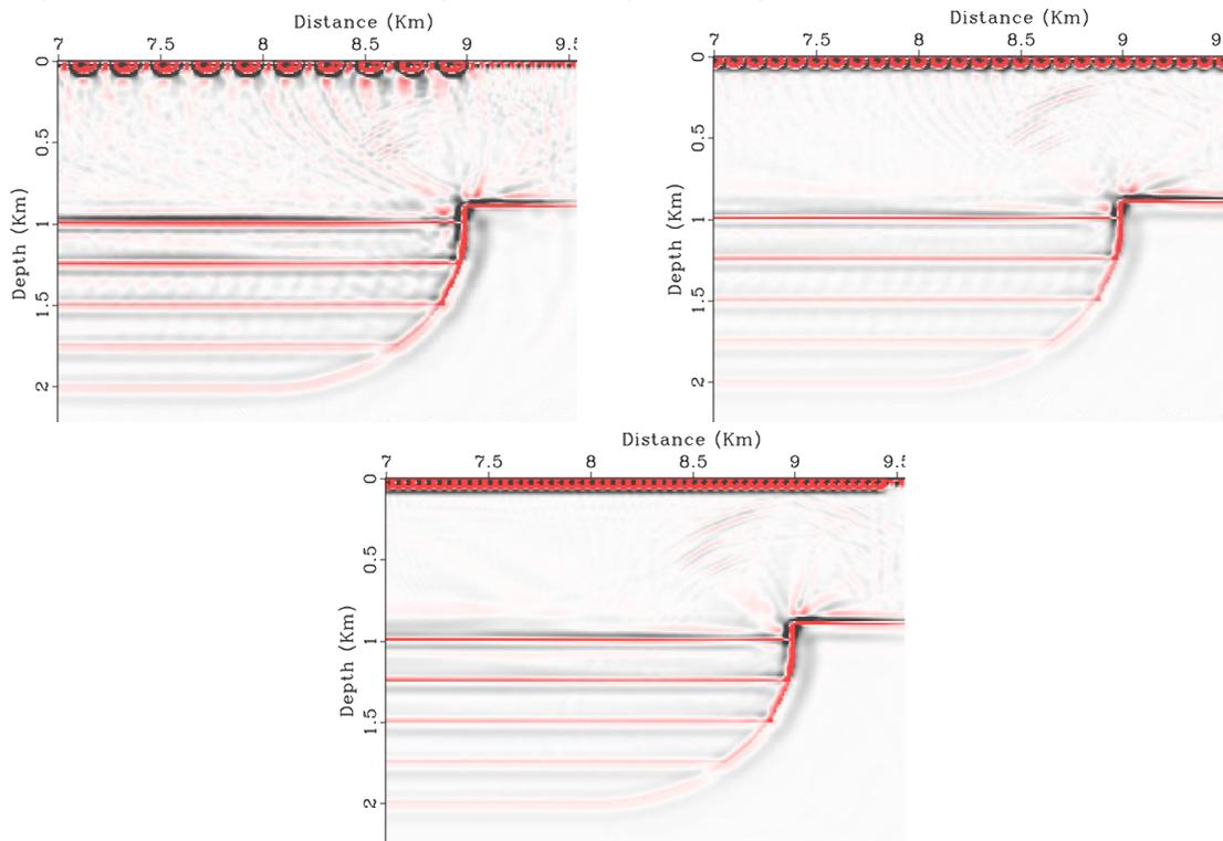
FIG. 2. RTM migrations of the selected surveys of Figure 1 right. Above are S1 with 15 shots and S2 with 45 shots. Below is S3 with 96 shots.
