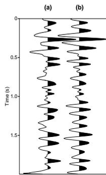
**Figure 3** Drill bit source signature. a) True and b) Estimated source signatures.
