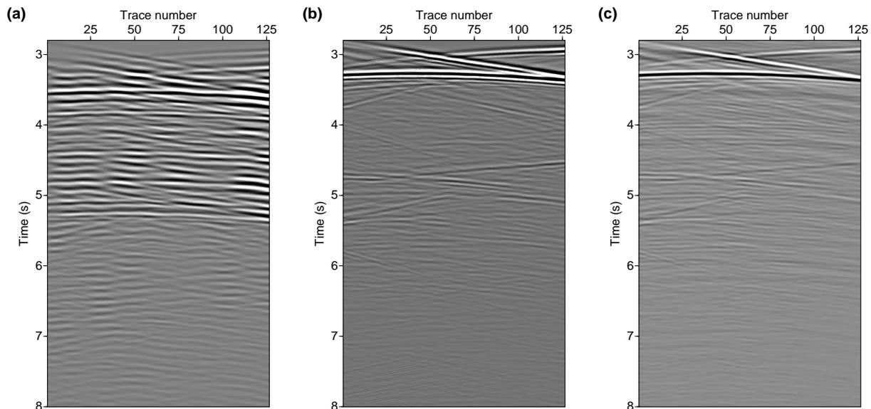
**Figure 2** Windowed version of SWD data. a) SWD shot gather. b) True drill bit source removed data. c) Estimated drill bit source removed data.
