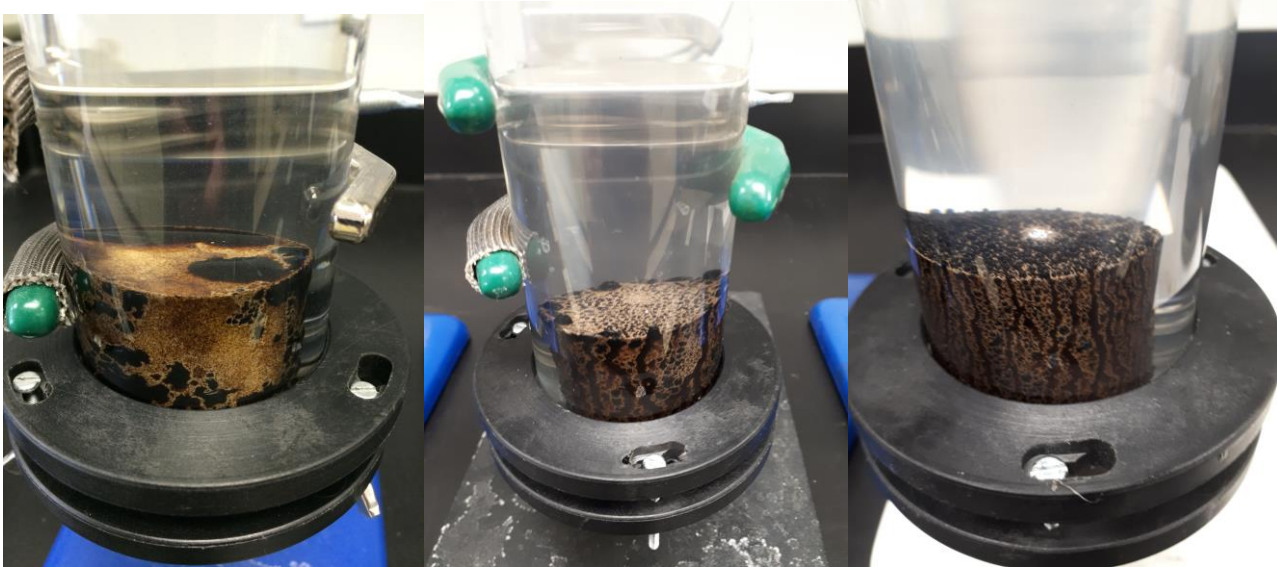
Area of oil drainage increased in core sample when exposed to different surfactants: Blank (Left), synthetic sulfonate (middle) and nano-molecule surfactant (right)
