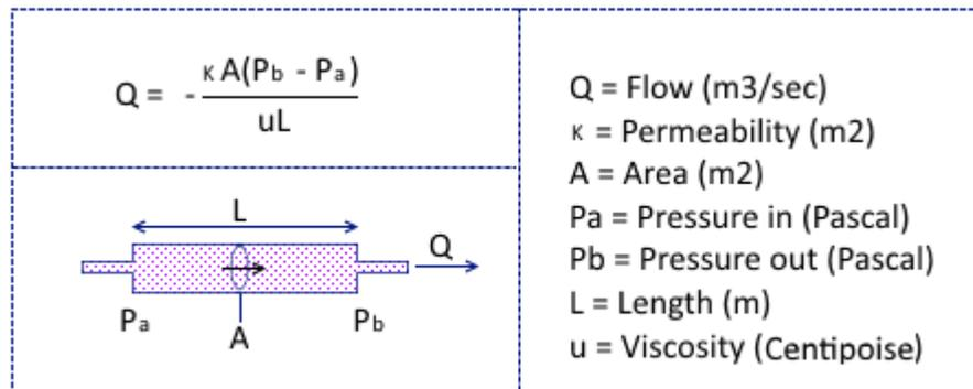
Increasing permeability of the formation with fractures will increase the flow rate of fluid in/out of the formation. Further promotion of fluid flow occurs by adding a time-released breaker which lowers the fluid viscosity, as a thinner fluid in the formation is transported faster than thicker fluids, with all other parameters being equal. All fluids are designed and tested to be compatible with:
