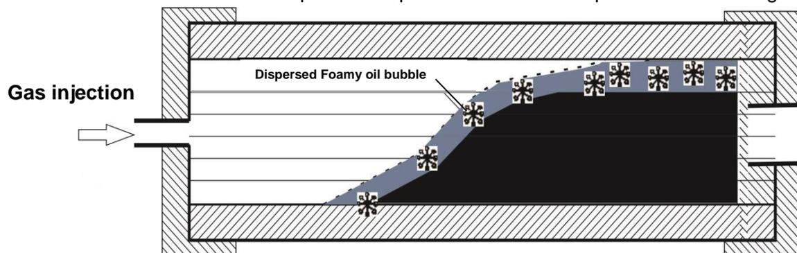
Figure 1. Displacement process of foamy oil after gas injection in heavy oil reservoir
