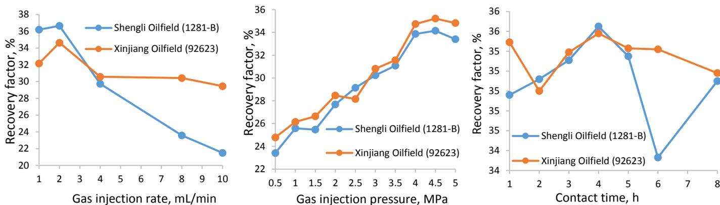
Figure 5. Oil recovery factor versus gas injection rate, gas injection pressure and contact time
