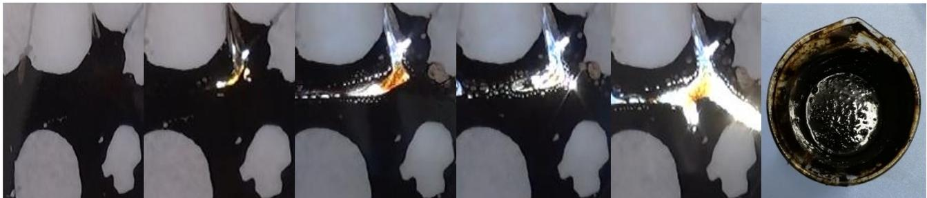
Figure 4. Pore displacement profile during gas injection process and produced foamy oil
