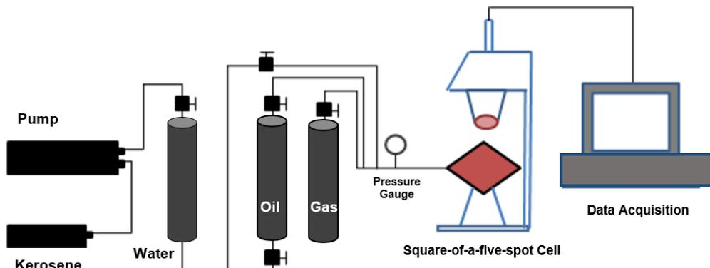
Figure 2. Experimental apparatus for foamy oil tests
