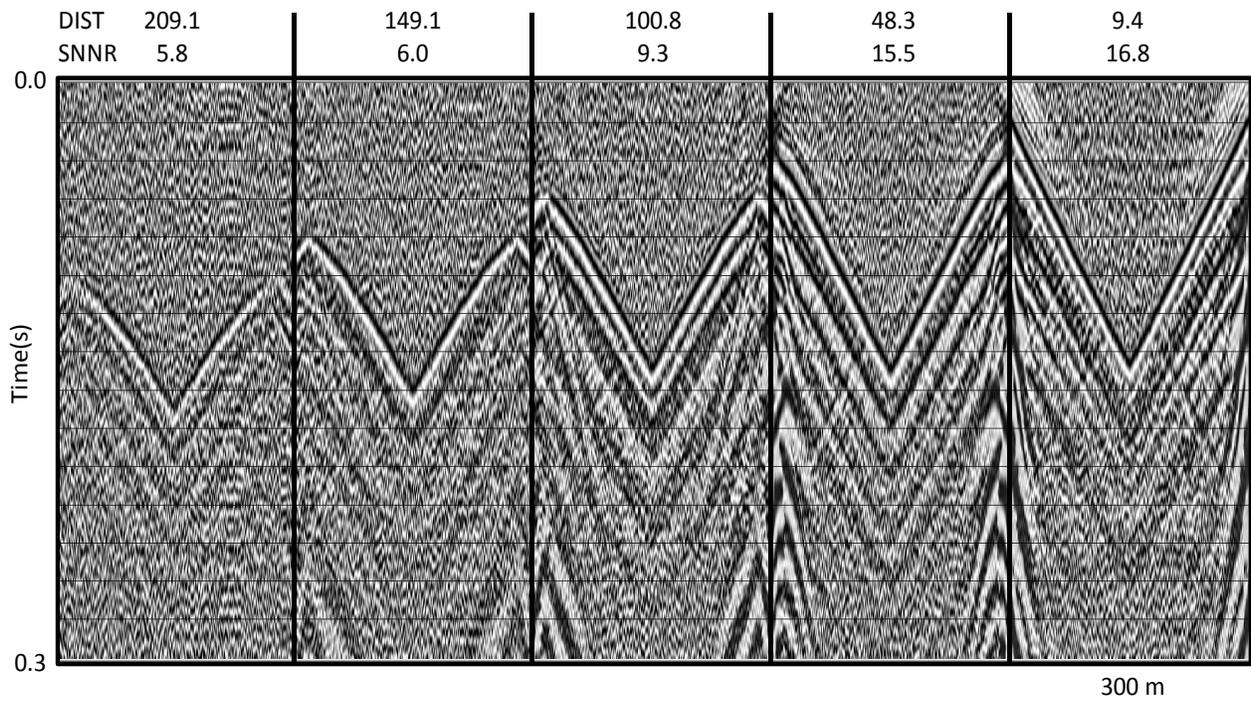
Figure 3. Source line 21 (July) correlated single sweeps recorded on straight fibre in geophysics well (black dots, Figure 1) with 10 ms AGC for display. Source distance from well decreases from left to right.
