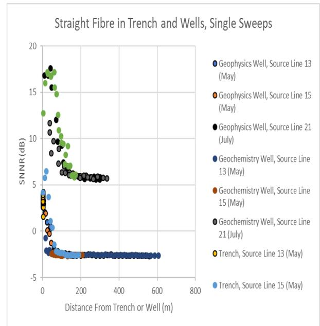
Figure 2. SNNR calculated for single-fold correlated gathers for all data recorded on straight fibre (top) and helical fibre (bottom) plotted against source distance from the fibre.
