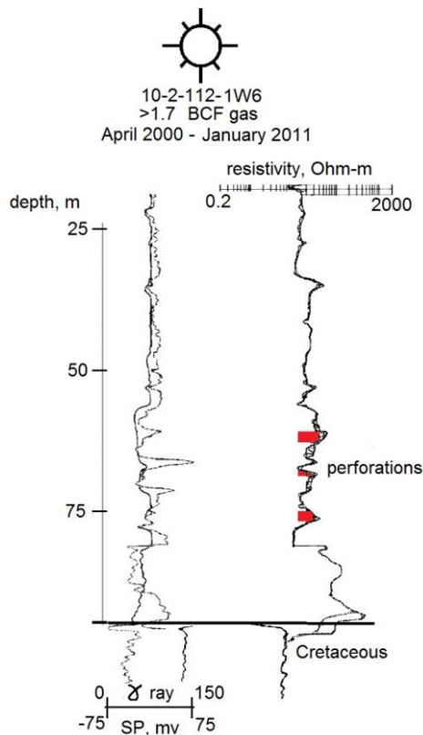
Figure 4. Resistivity well log from northern Alberta showing the productive sandstone stringers producing from glacial strata (modified from Pawlowitz, et al. (2003)).
