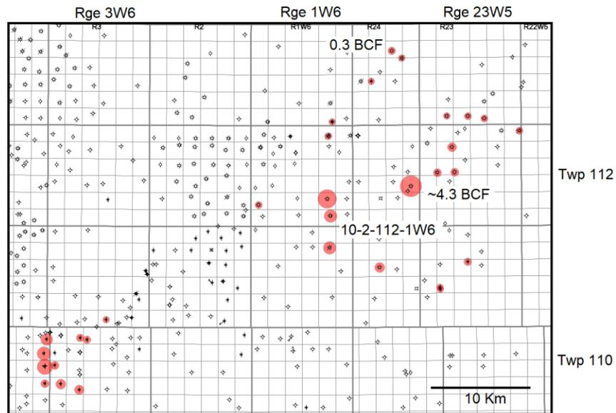
Figure 3. Well base map from northern Alberta showing natural gas production from ~30 wells. The resistivity log for 10-2-112-1W6 is shown in Figure 4.
