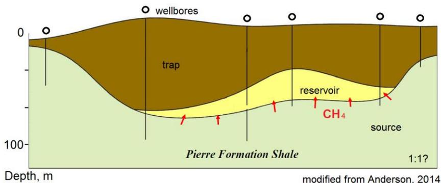
Figure 2. A six well cross section showing a glacial sandstone reservoir overlying Upper Cretaceous Pierre Shale and overlain by tite glacial sediments.
