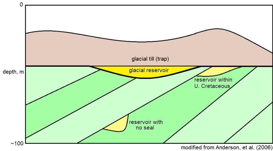
Figure 6. Cartoon sketch (modified from Anderson, et al., 2006) to show the angular unconformity between glacial sediments and Upper Cretaceous that may enhance hydrocarbon movement. Also, any reservoir in the Upper Cretaceous that is trapped by the fault geometry may be prospective for shallow gas.
