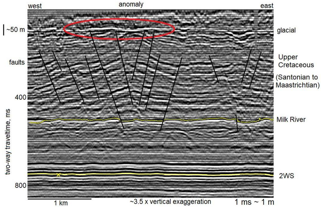
Figure 5. A 2-D seismic line from southeast Saskatchewan imaging highly faulted Upper Cretaceous strata above the Milk River (Santonian). These strata are unconformably overlain by glacial till that may contain lenses of porous and permeable reservoir sands as circled in red.
