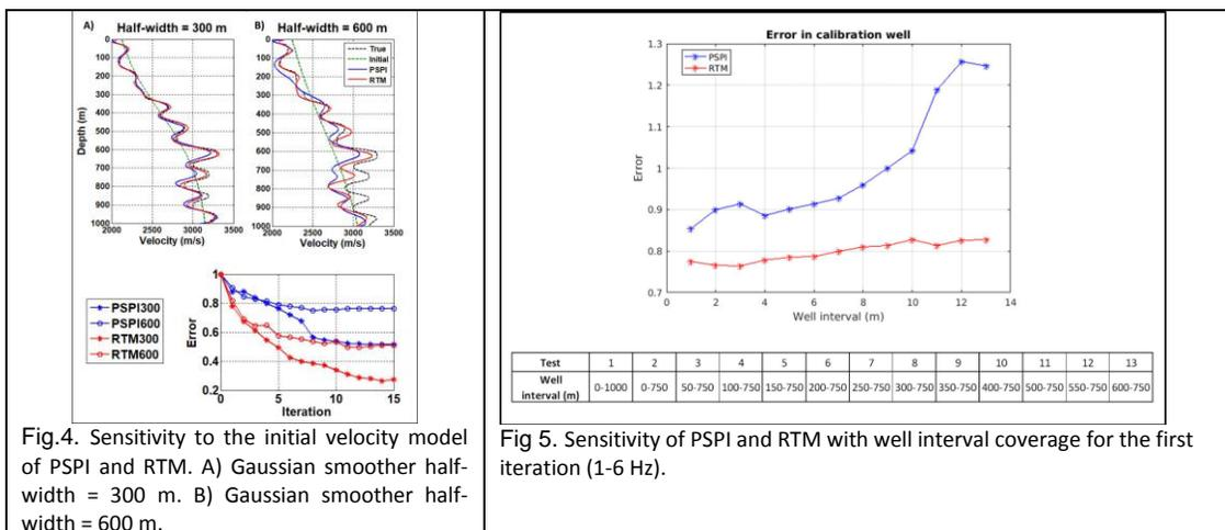
Fig.4. Sensitivity to the initial velocity model of PSPI and RTM. A) Gaussian smoother half-width = 300 m. B) Gaussian smoother half-width = 600 m.
