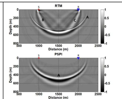
Fig. 2. PSPI and RTM applied to the 1000-m offset trace of figure 1.
