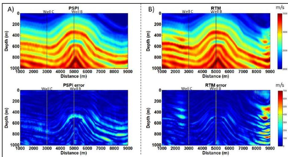
Fig. 3. Final inverted model after 15 iterations: A) PSPI and B) RTM.
