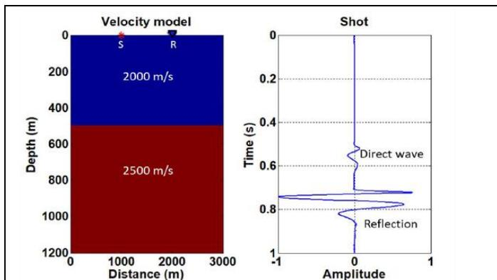
Fig. 1. Seismic trace generated by finite-difference modelling through a single interface model.
