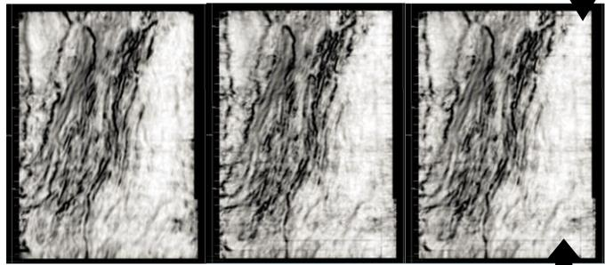
Figure 7: Similarity time slice along green horizon. Far left: PSTM. Middle: 5D PSTM. Far right: 5D PSTM with prior 2D interpolation. Note the east-west artifacts (indicated by the arrows) on both 5D volumes not seen on the PSTM volume. These artifacts are also not visible on the amplitude time slices of Figure 6.
