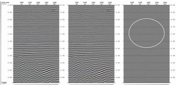
Figure 1: 5D ALFT leakage stack test displayed in grey scale to clearly see the leakage. Far left: input data. Middle: 5D interpolation. Far right: leakage. Leakage is very minimal and mainly limited to the shallow section as indicated.
