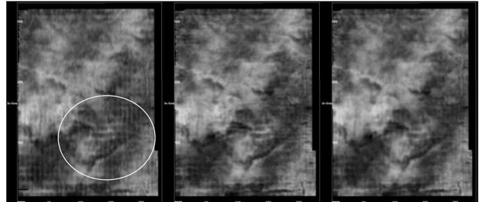
Figure 4: Amplitude time slice 850ms. Far left: PSTM. Middle: 5D PSTM. Far right: 5D PSTM with prior 2D interpolation. Note the clearer image of 5D PSTM over PSTM. Note also the clearer image of 5D PSTM with prior 2D interpolation over 5D PSTM as indicated by the circle.
