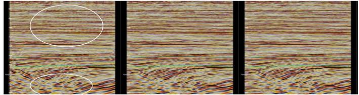
Figure 2: Example inline section. Far left: PSTM. Middle: 5D PSTM. Far right: 5D PSTM with prior 2D interpolation. Note the superior shallow continuity and fault imaging in the 5D sections as indicated by the circles.
