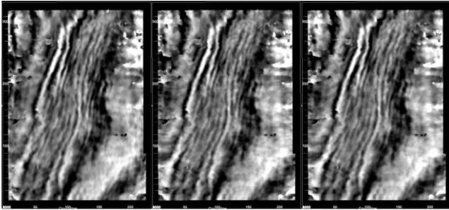
Figure 6: Amplitude time slice along green horizon. Far left: PSTM. Middle: 5D PSTM. Far right: 5D PSTM with prior 2D interpolation.
