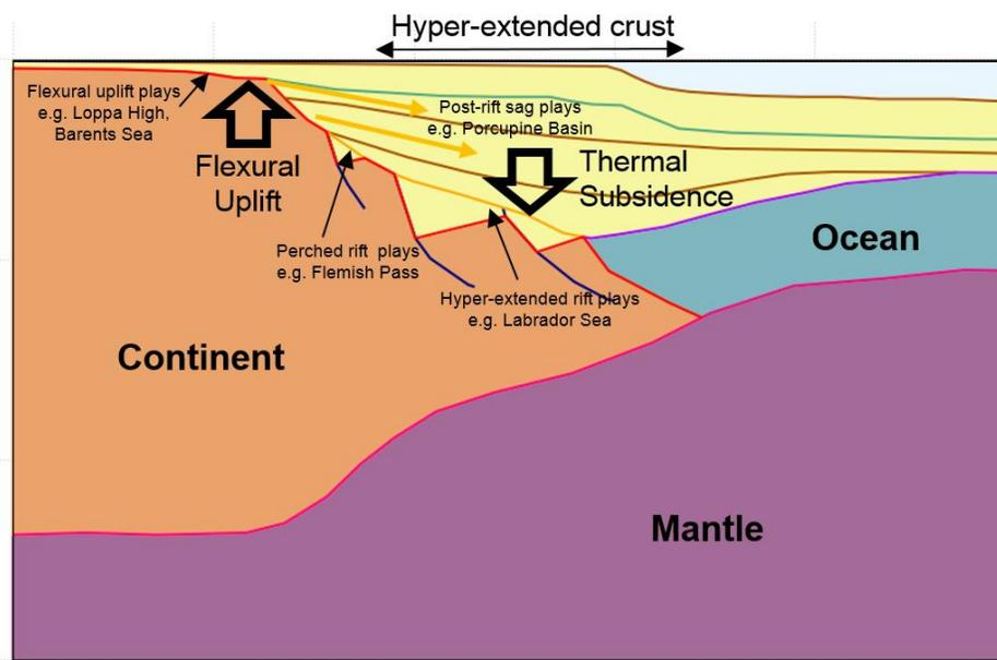
Figure 2: Schematic cross section of a hyperextended margin showing some examples of play types associated with this structural setting.
