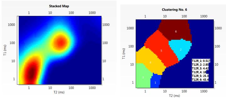
The T1-T2 map from the saddle point tool reveals multiple poro-fluid components that are less than 20 ms. The Meramec formation does not contain any significant kerogen content, nor is bitumen expected, so these three components have been interpreted as various waters. Had kerogen or bitumen been present, the high T1-T2 ratio component would have been identified as bound hydrocarbon, increasing the bulk volume hydrocarbon over
