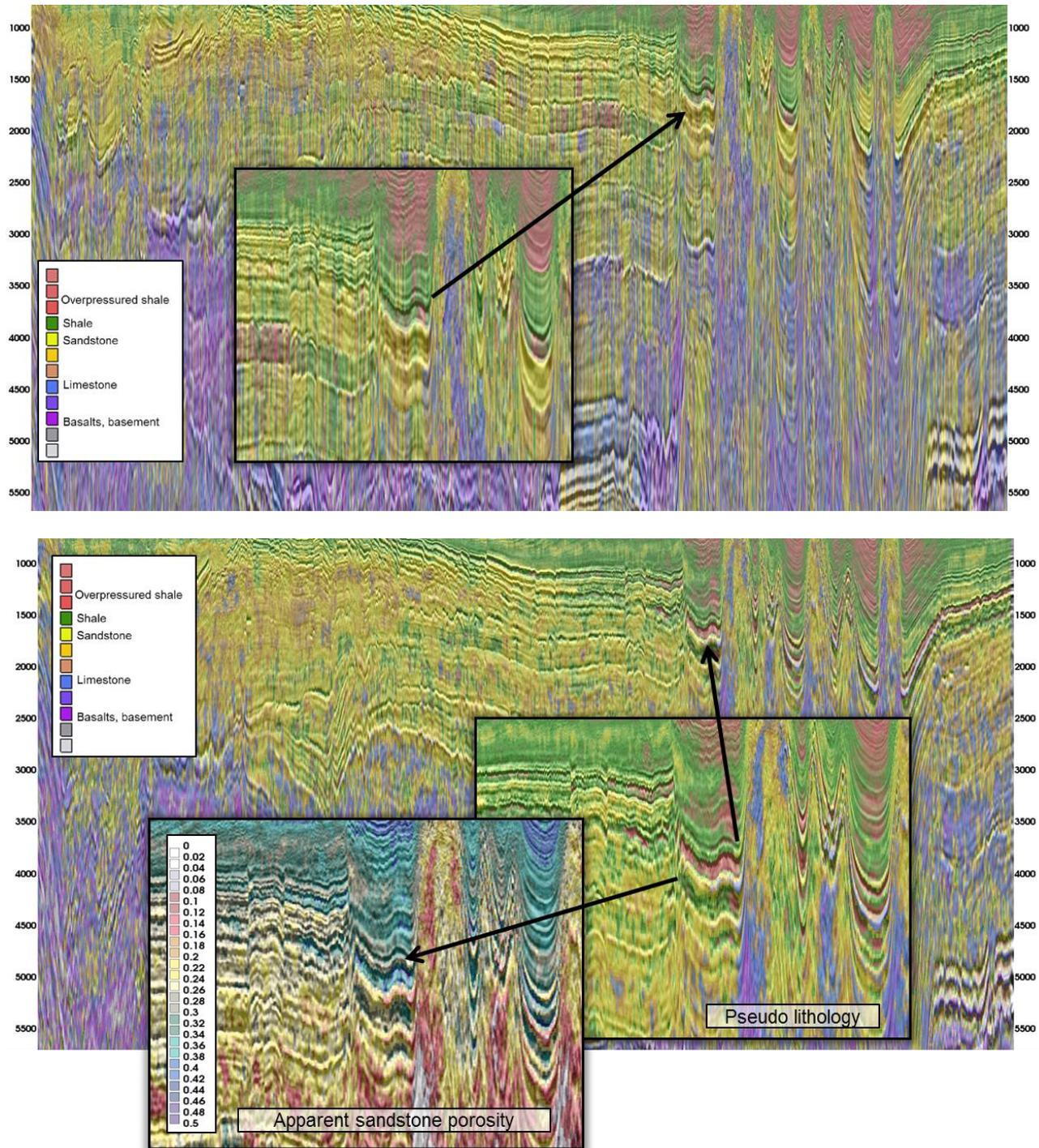
**Figure 1** Pseudo Lithology from stacking velocities (top), Pseudo Lithology and apparent sandstone porosity from HighRes velocities (bottom). The HighRes velocities resolve a thin hot shale layer (red), and are less noisy. There are sandstones with reservoir potential below the hot shale, the apparent sandstone porosity indicates porosities between 20% and 25% in these, which is very acceptable for exploration.
