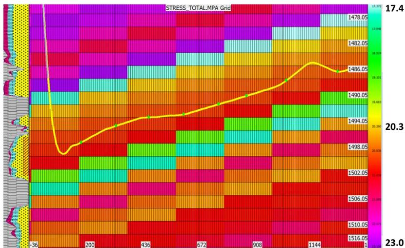
Figure 2: Geological structure of the Bakken Formation in a horizontal well in the Viewfield area. Colours represent minimum horizontal stress magnitude, yellow line denotes well trajectory and green squares denote perforations.
