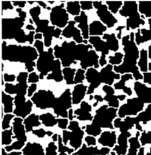
(a) CT scan image of Berea sandstone
