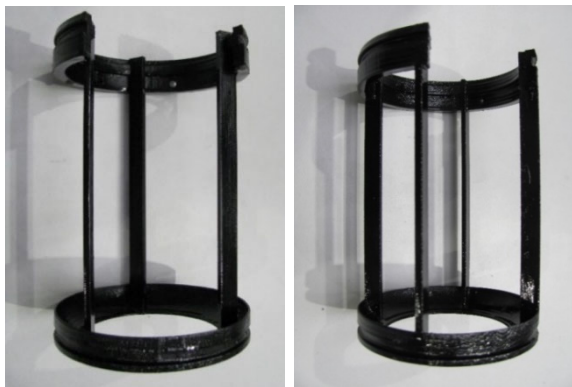
Fig. 2 - 3D printed baffles in titanium. On the left-hand side: three baffle set far from the tank wall and on the right-hand side: four baffle set adjacent to the tank wall.
