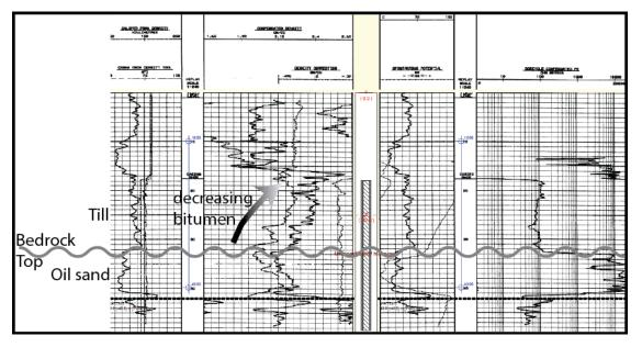
Fig. 3 Example (8-7-98-6W4) of till containing high oil sand at base, and progressively less from contact. Rather than an abrupt shift in the neutron curve, the shift is more gradual as the concentration of bitumen decreases up hole.
