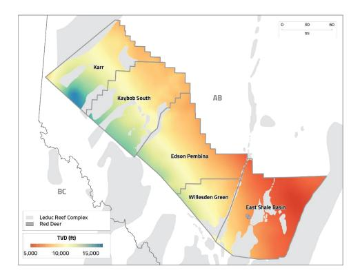
Figure 1 | Duvernay Play With Sub-Basins and Structure Map, Highlighting Shallow Nature of the East Shale Basin.
