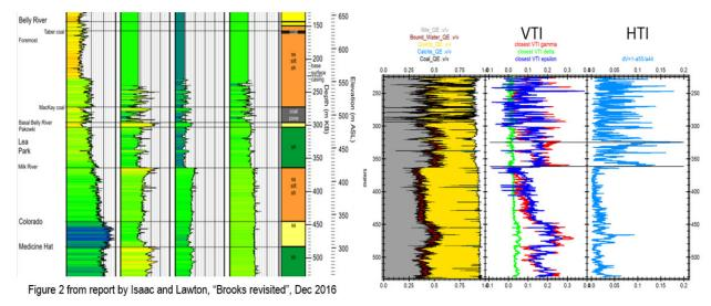
Figure 1. Lithology at the CAMI site (left) and petrophysical volumetric analysis with sonic anisotropy logs.
