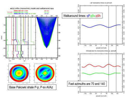
Figure 2. Upscaled monoclinic model with depth-dependent fast azimuth (upper left) and qP, qSv qSh rays from surface to a receiver at depth z=400m below the orthorhombic Lea Park formation. Lower left: Right: walkaround qP, qSh and qSv times for a circle at radius r=500m.
