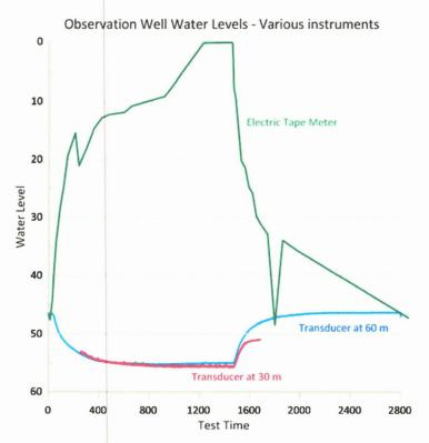
The top of water column measurement (green) provides no usable data with respect to aquifer interpretation whereas the two pressure transducers show more typical pumping test results. The transducers do show some deviations between each other due to increasing gas flow rates during the pumping portion of the test. The transducer at 30 m (red) shows "noisy behavior" which upon closer inspection is likely a result of bubbly or slug flow conditions.
