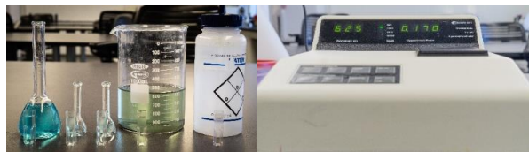
Figures 2 & 3: Measuring copper concentration using UV-vis spectroscopy
