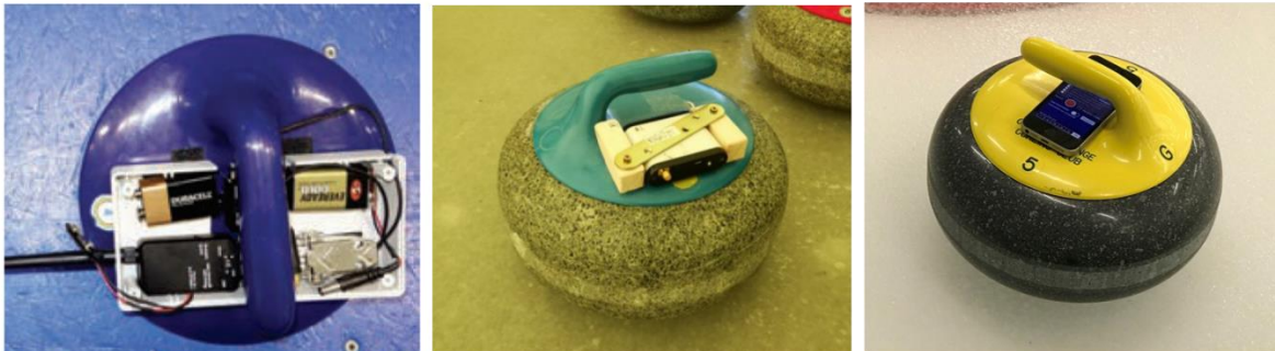
Figure 2. Three IMU (inertial measurement unit) systems. Left: Lozowski et al. (2014), middle: Djikowski (2018); right: the iPhone SE with Sensor Play app used here.
