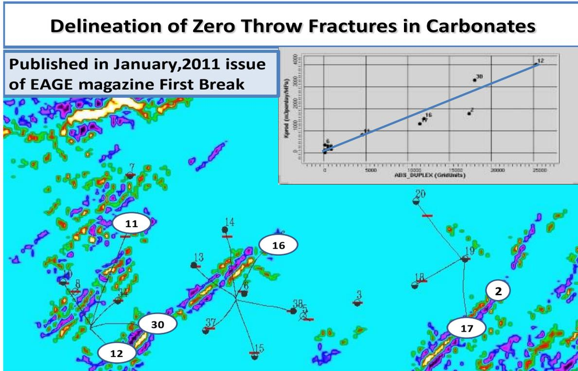
Figure 2: This is a DWM amplitude map that has delineated the location of permeable fracture systems within an accuracy of 25 meters. Note that the graph of DWM amplitudes versus measured permeability (total fluid flow rates of water plus oil measured at each producing well) is linear. This indicates that DWM provides a reliable predictor of fluid content and permeability within the fault/fracture system.
