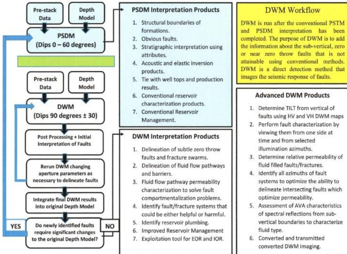
Figure 3: this workflow illustrates the function the DWM process relative to conventional PSTM and PSDM products.
