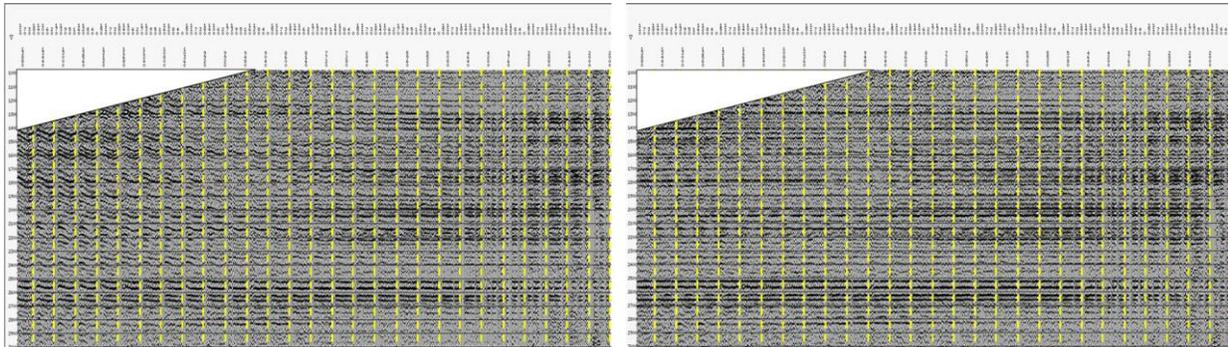
Figure 2: COCA cubes showing azimuthal velocity variations (left) and after application of azimuthal velocities (right).
