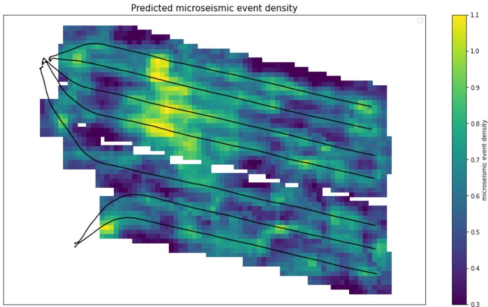
Figure 5. Predicted microseismic event density for a set of new wells
