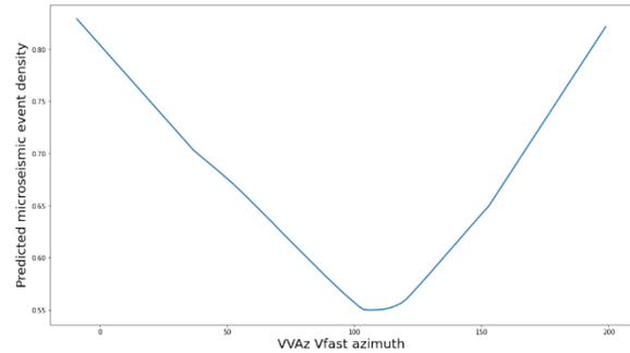
Figure 7c. VVAz fast velocity azimuth versus microseismic event density
